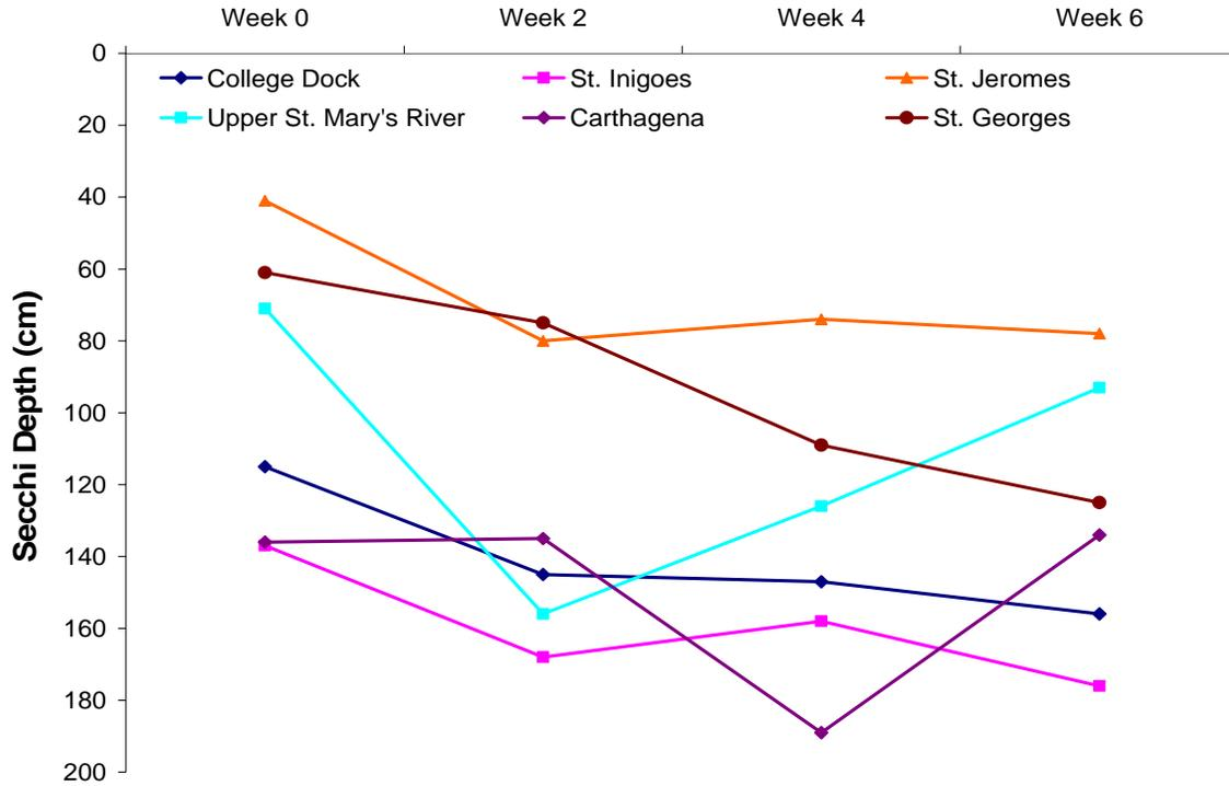
Figure 5. Secchi disk depth measured at the six study sites biweekly over the course of six weeks, October - November 2009.
